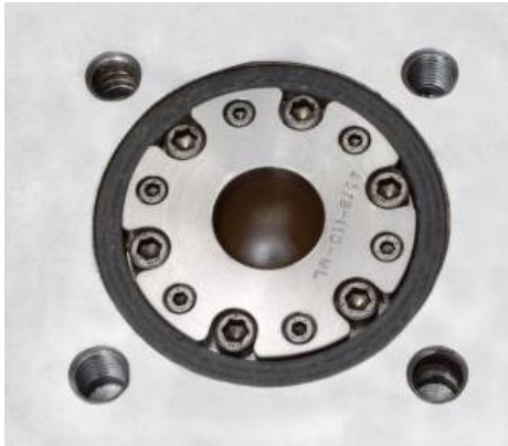
Rupture Disc Assembly embedded in the Pressure Plate
